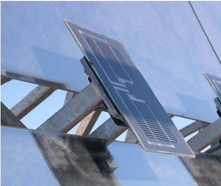
Sun sensor made of two photovoltaic cells (developed by FLAGSOL)
