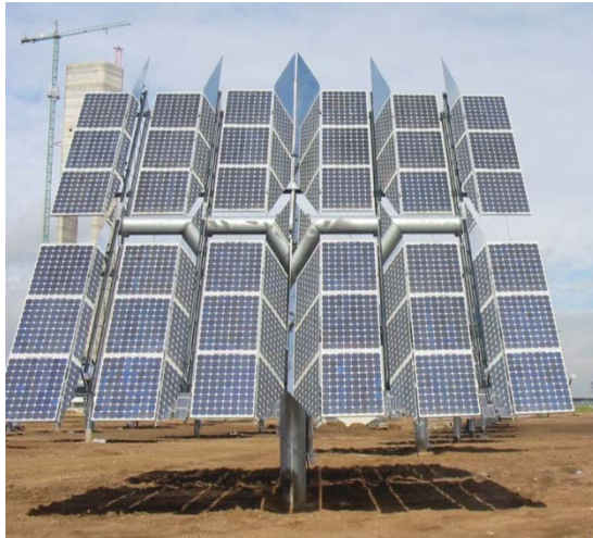
PV panels using flat mirrors for solar concentration
